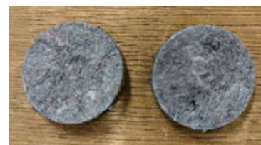
a. Felt laminated with CNF
