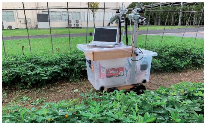
Figure 6. Developed pesticide spraying robot
